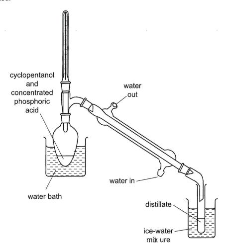
2 The distillate has an aqueous layer and an organic layer. The student purifies the cyclopentene from the distillate.
