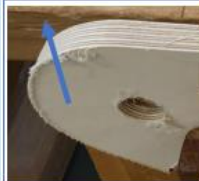
An example of pieces after routing. Filing should be done in the direction of the arrow to avoid chunks of ply being torn away from the piece.
